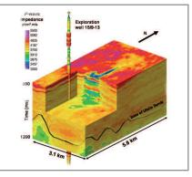
3D view of the distribution of P wave impedance obtained following seismic inversion of data acquired in 2006.  $CO_2$  is identified by lower impedance values (blue and green colors) inside the reservoir (as per Clochard et al. First Break 2010).
