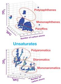
3D chromatograms produced by analysis of a vacuum distillate by SFC / GC2D-HT coupling.
