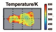
Image of the temperature in a non-reactive diesel jet obtained by laser induced fluorescence.
